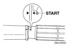
4. Pull out / turn the choke knob fully. Place the choke knob back in to the second or third position to warm up the engine after starting. When the engine has fully warmed up, replace the choke knob back in to its home position.
